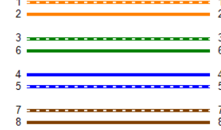
Schema collegamenti (T568B)
